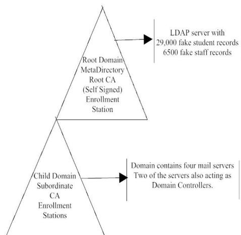
Figure two. A topological diagram of trial one as seen from a Windows forest perspective.
