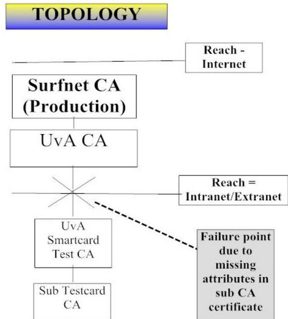
Figure 1. Topological diagram of planned Infrastructure and the final outcome due to certificate revocation issues.
